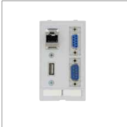
RJ45; USB; SUB-D9; SUB-D9 1 x RJ45, 8-pole. Metal, CAT5e (socket/socket); 1 x USB (socket/socket) Type A; 1 x SUB-D9 (socket/socket); 1 x SUB-D9 (pin/pin)
