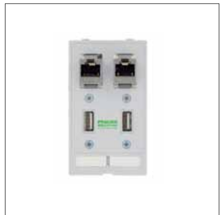
RJ45; RJ45; USB; USB (type A) 2 x RJ45, 8-pole. Metal, CAT5e (socket/socket); 2 x USB (socket/socket/0.7 m cable) type A
