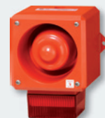
YL50 Industrial Combination Signal 110 dB (A) / 5 Joule CPR - EN54 Part 3 & 23 certified
